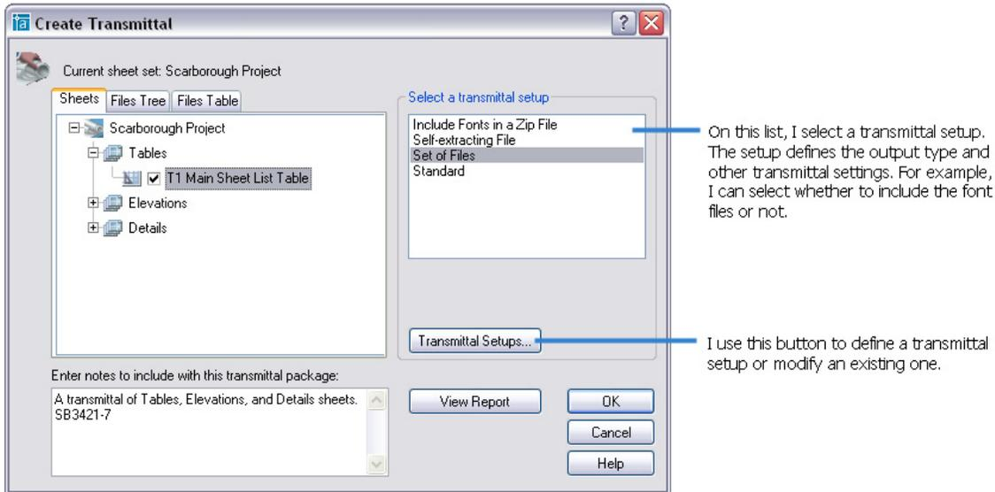
To create the transmittal I, click the Tables heading, and then press the CTRL key to select the Elevations and Details headings. I right-click one of the selected headings, and click eTransmit. In the Create Transmittal dialog box, I select one of the saved transmittal setups, and then click OK.
